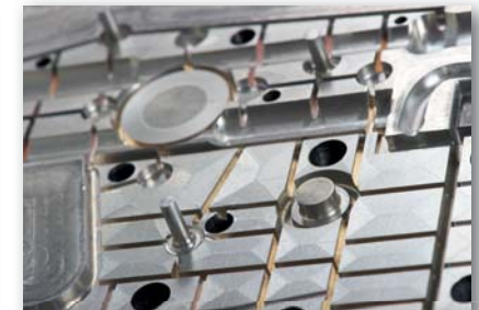
RAPID TOOLING Milled tooling inserts and near-series prototypes
