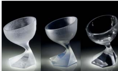
TRANSPARENT PIECES Surface finishing by means of sanding and polishing
